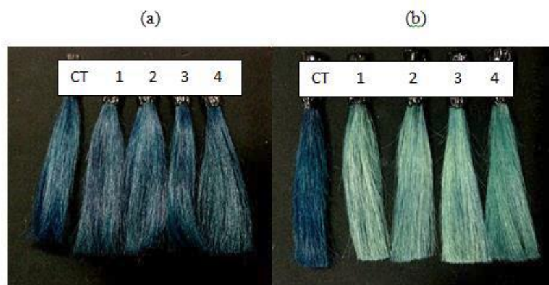
Figure 6 Blue hair dye before and after 10 washing process with each shampoo formulation (CT = control, 1 = SLES shampoo, 2 = SLS shampoo, 3 = SLES with NaCl shampoo and 4 = Sulfate free shampoo), (a) blue hair after bleaching and dyeing (b) blue hair dyed after 10 washes.
