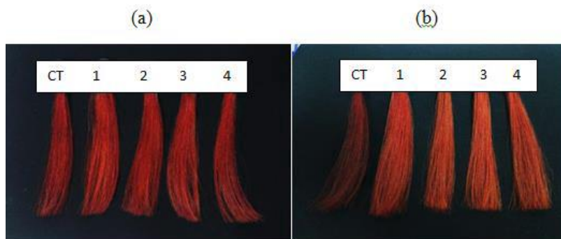
Figure 5 Red hair dye before and after 10 washing process with each shampoo formulation (CT = control, 1 = Sulfate free shampoo, 2 = SLS shampoo, 3 = SLES shampoo and 4 = SLES with NaCl shampoo), (a) red hair after bleaching and dyeing (b) red hair dyed after 10 washes
